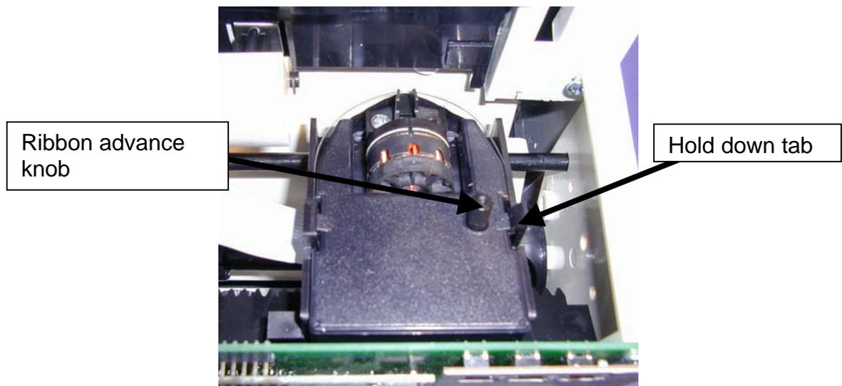
Note: If the ribbon is not completely over the print head the resulting print will show incomplete characters. If the ribbon cartridge is not completely snapped in the holder the resulting print will be increasingly lighter.
