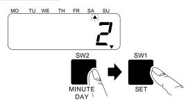
Press the [SW2: MINUTE/DAY] key until the correct number appears. The repeat times can be selected 0 to 9. Press the [SW1: SET] key after checking the desired number on the LCD.
