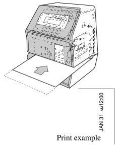
PLEASE NOTE: If a time card is inserted and removed too quickly, the print head will move, but no imprinting will occur. This feature is designed to protect and maintain the life of your printer. Please hold the time card in the recorder until the print head movement is complete.
