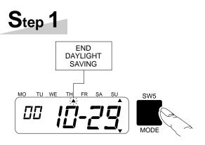
Press the [SW5: MODE] key four times, the "END DAYLIGHT SAVING" arrow flashes.
