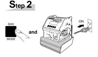
Plug the AC cord into the AC outlet while pressing the [SW5: MODE] key. Then "0" is mentioned on the LCD.
