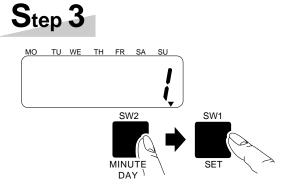
Press the [SW2: MINUTE/DAY] key until the correct number on the LCD.
