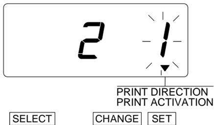
In case of the example, press the **CHANGE** button to set at "2". And then press the **SET** button.
