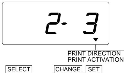
In case of the example, press the **CHANGE** button to set at "3". And then press the **SET** button.
