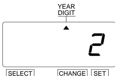
In case of the example, press the **CHANGE** button to set at "2", and then press the **SET** button.
