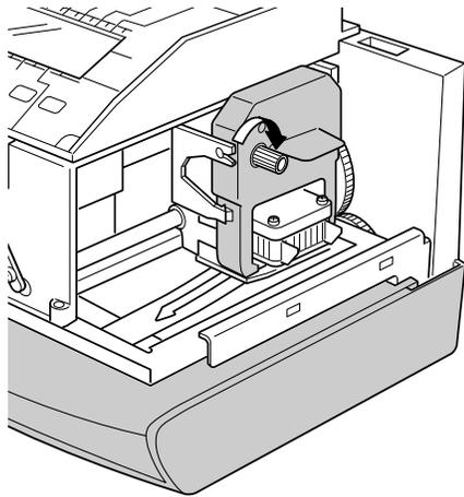
Turn the knob of the cassette in the direction of the arrow to tighten the ribbon.
