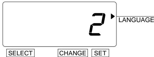
In case of the example, press the **CHANGE** button to set at "2". And then press the **SET** button.
