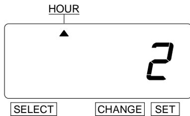
In case of the example, press the **CHANGE** button to set at "2". And then press the **SET** button.
