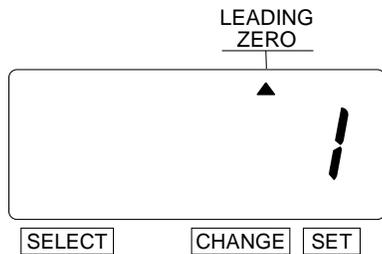
In case of the example, press the **CHANGE** button to set at "1". And then press the **SET** button.
