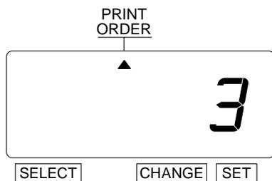
In case of the example, press the **CHANGE** button to set at "3". And then press the **SET** button.
