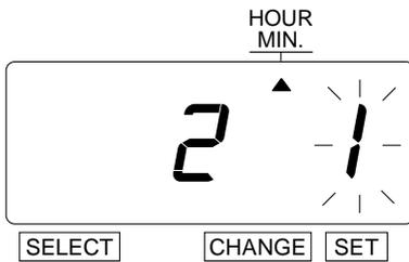
In case of the example, press the **CHANGE** button to set at "2". And then press the **SET** button.
