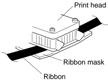
**NOTICE:** Install the cassette so that the ribbon is between the print head and the ribbon mask. Printing will not come out properly if the ribbon is placed behind the ribbon mask.
