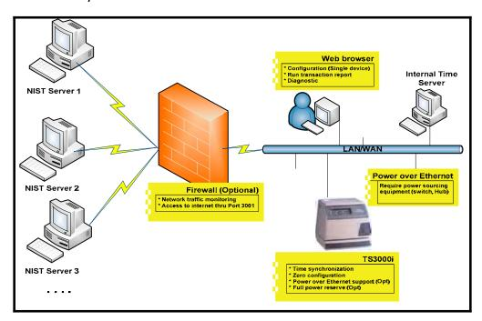
Figure 1-1: TS-3000 Web Clock Time Synchronization
