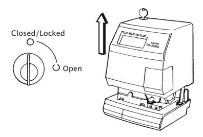
Figure 2-2: TS-3000i Web Clock Cover Removal
