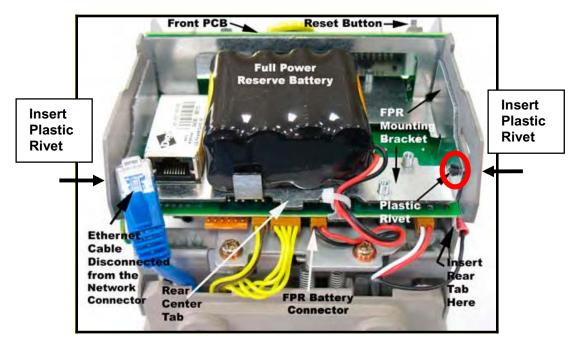
Figure 2-7: TS-3000i Clock Rear View
