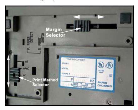
Figure 2-17: TS-3000i Printer Adjustment
