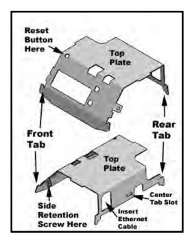
inserted into its side retaining slots on the right and left sides of the main clock frame (see *Figure 2-6*).
