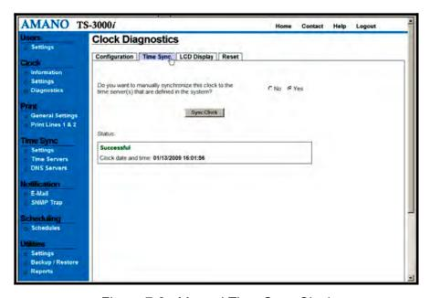
Figure 7-2: Manual Time Sync Clock
