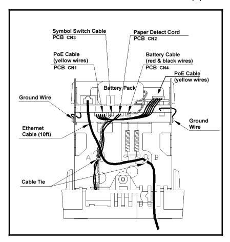
Figure 2-13: Rear View Showing PoE & FPR Cables/Connections
