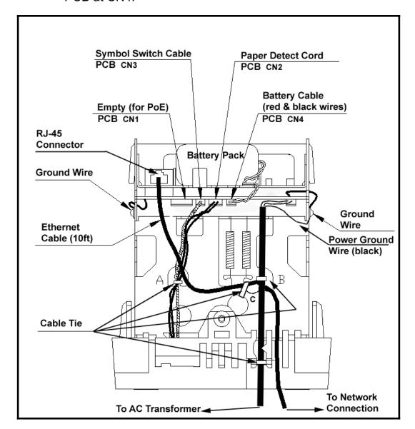
Figure 2-8: Rear View Showing Cable/Connector Location
