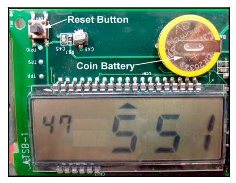
Figure 7-8: Reset Button Location
