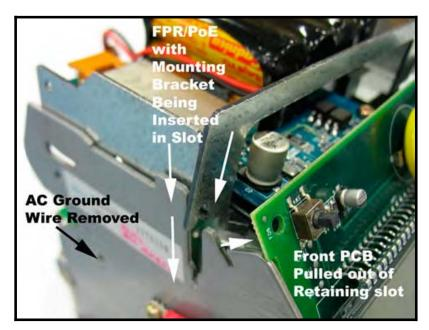
Figure 2-11: Front PCB & Mounting Bracket
