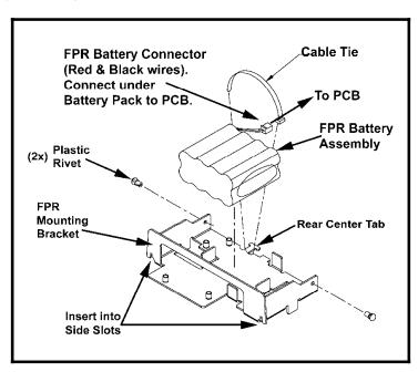
Figure 2-5: FPR & Mounting Bracket
