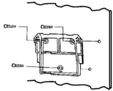
Step 4. Align the TS-3000i Web Clock with the hooks on the mounting plate. Press down and toward the wall until a "CLICK" is heard. Replace the cover, lock it and remove the key. Your TS-3000i Web Clock is now wall mounted.
