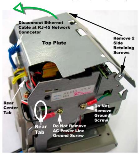
Figure 2-4: Top Plate Removal
