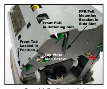
Figure 2-9: Top Plate Installed
