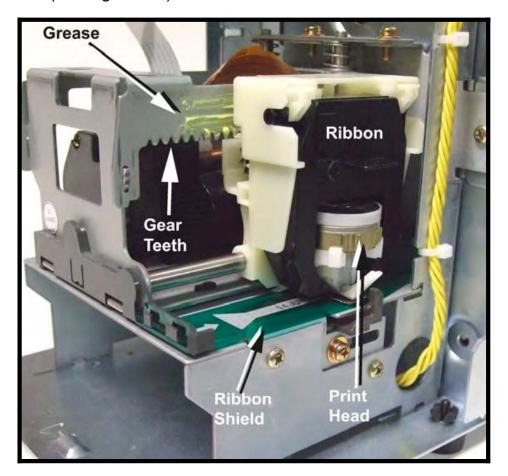
Figure 7-9: Ribbon Carriage Grease
