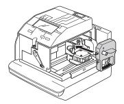
Place the cassette inside the time recorder as shown in the figure. Push the ribbon until it snaps into position. Turning the knob on the ribbon cassette may make installation easier.
