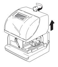
Unlock the key and remove the cover.
