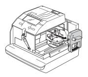
Hold the ribbon cassette by its tab and pull straight out to remove it.
