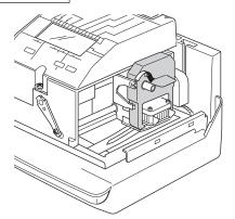
Turn the knob of the cassette in the direction of the arrow to tighten the ribbon.
