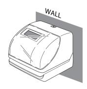
Install the supplied wall-mount screws into a wall by using the template. Be sure to keep about 6mm(1/4") of the screw head away from the wall. The recommended height from the floor to the bottom of the ES700 is 45".
