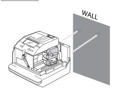
Unlock the key and remove the cover. And then hang it on the wall.
