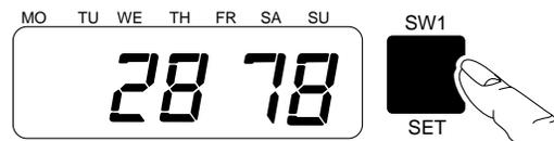
Press the [SW1: SET] key. "▼" located right-below on the LCD will disappear that confirms password setting.
