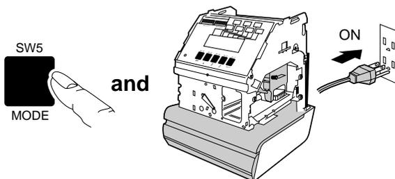
Plug the AC cord into the AC outlet while pressing the [SW5: MODE] key.
