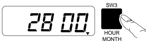
Press the [SW3: HOUR/MONTH] key and assign the desired numbers to first two digits.
