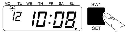
Press the [SW1: SET] key after checking the desired time appears on the LCD.
