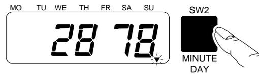
Press the [SW2: MINUTE/DAY] key and assign the desired numbers to the last two digits.
