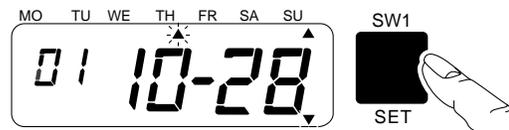
Press the [SW1: SET] key after checking the desired year, month and day on the LCD.
